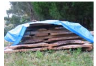
Above: Camphor on site is felled and sawn into slabs on Lot 4, to be used once it's seasoned.
